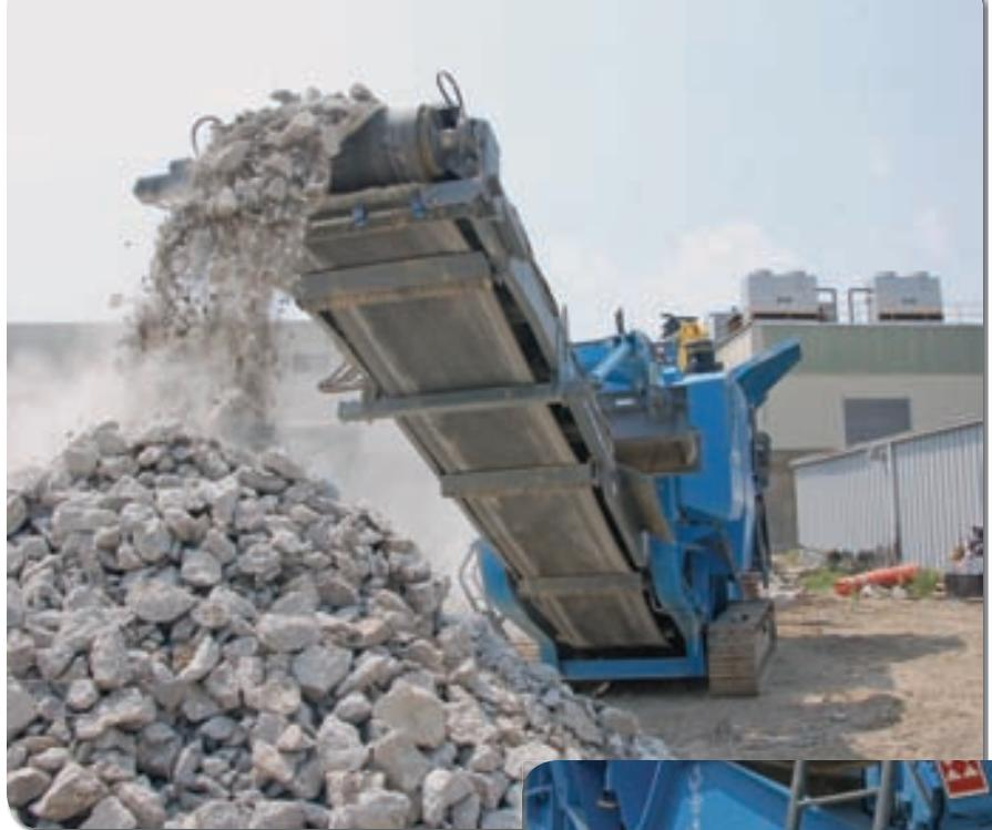
Above: High-performance Terex Pegson XR400 can crush up to 400 tons an hour.
